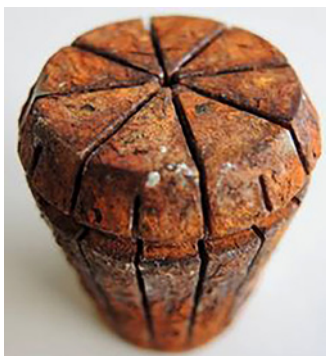
Standard ER Collet Material: Conventional Spring Steel
