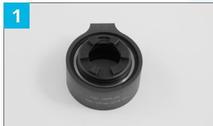
Mark the position of the inner part to outer ring.
