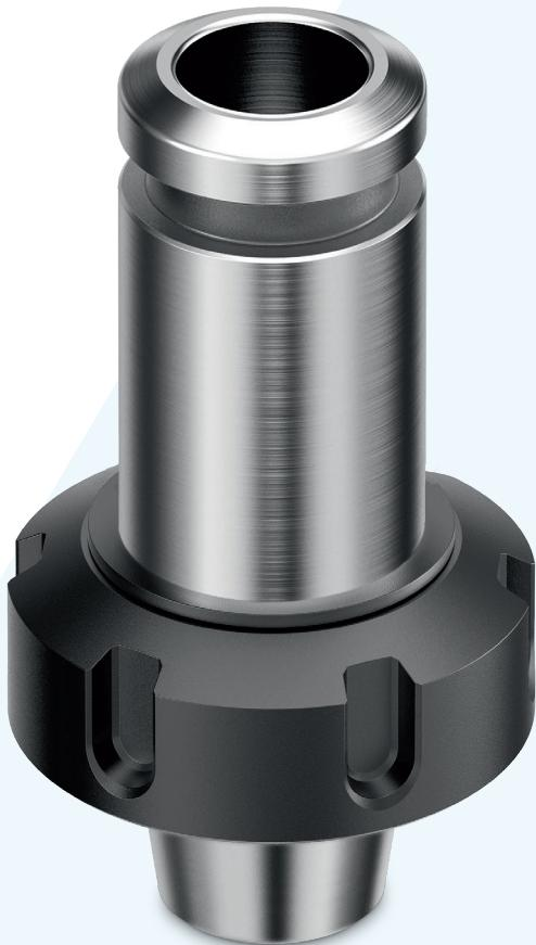
**What is it?** The swissQuick ER-to-PG adapter is a short "mini-holder" with a solid ER body profile on the back, with a powRgrip collet cavity on the front. This unique design allows for quick tool changes with an ER fixture while still receiving the benefits of the powRgrip system.
